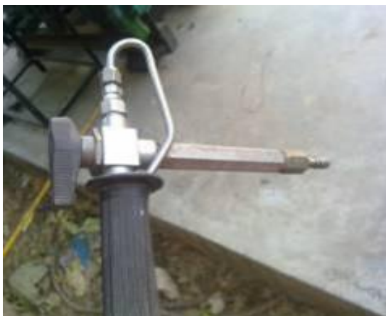
(a) Upgraded and compressed biogas dispensing nozzle (Source: Author)
