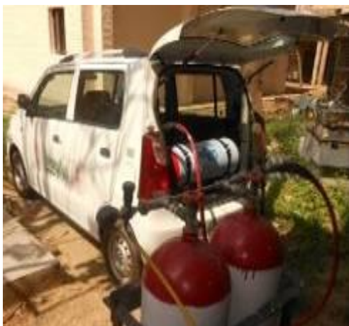
Figure A7. 2-cylinder cascade system for on-site dispensing of upgraded biogas at IIT Delhi
