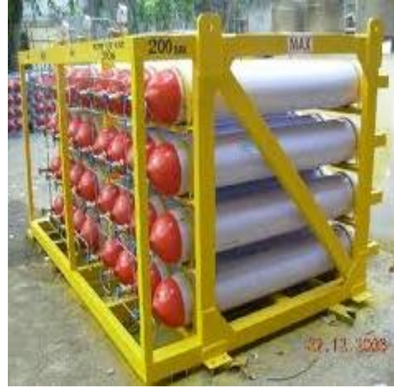
(b) Cascade of cylinders for storage and transportation of upgraded and compressed biogas
