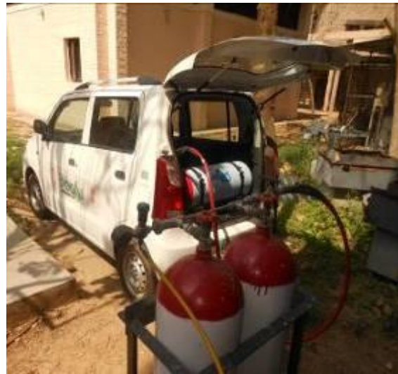
(c) and (d) Trial runs of biogas as a transport fuel in natural gas vehicle
