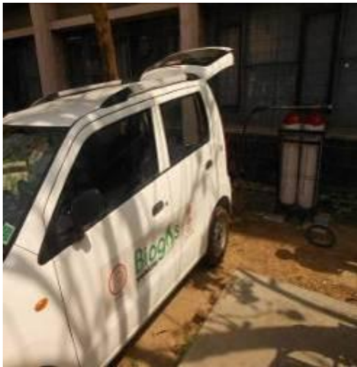
(c) and (d) Trial runs of biogas as a transport fuel in natural gas vehicle
