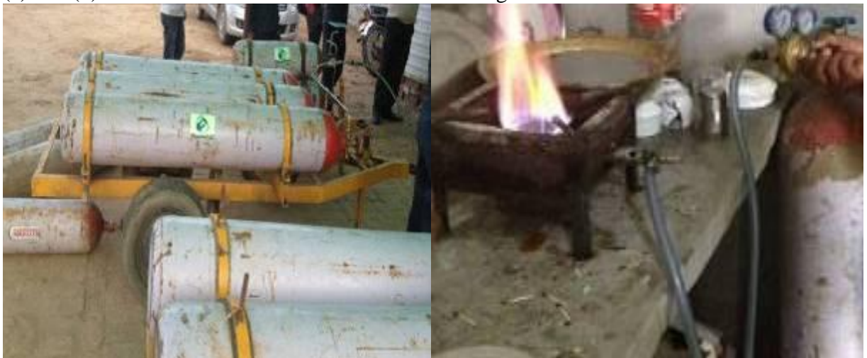
(c) Bottling of upgraded biogas in CNG cylinder cascade (d) Bottled biogas being used for cooking
